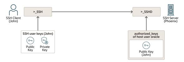
SSH user keys of the SSH client *John* are created by *John* or by an administrator. The keys are stored on the SSH client host. *John*'s public key is added to the authorized\_keys file of the *oracle* user on SSH server *phoenix*. *John* can now initiate connections as *oracle* to SSH server *phoenix*. However, connections as other users like opc on *phoenix* is denied since *John*'s public key does not exist in the authorized keys file of opc
