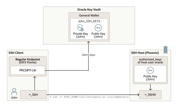
Figure 15-6 Centralized-SSH-User-Key-Management
