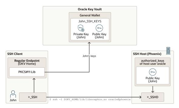
Figure 15-6 Centralized-SSH-User-Key-Management
