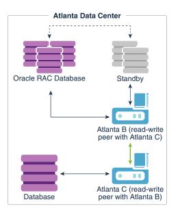
Figure 3-1 Oracle Key Vault Multi-Master Cluster Deployment in Single Data Center
