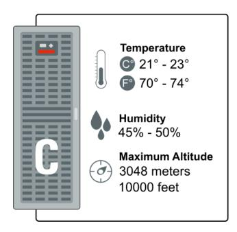
The following table lists the temperature, humidity and altitude requirements for Exadata Cloud at Customer.
