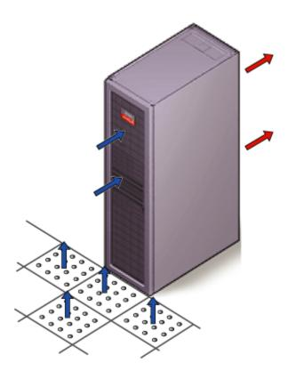
The following table lists the cooling requirement for each Exadata Cloud at Customer X6 rack:
