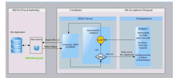
This image shows the process flow for sending and receiving the intermediate (second) SML file:
