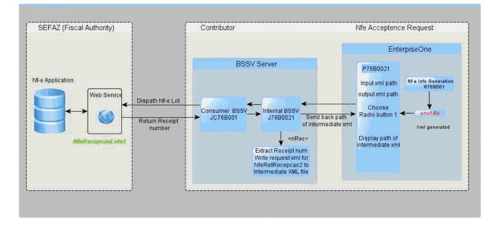
This image shows the process flow for sending and receiving the initial XML file:
