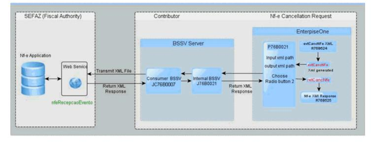
When you transmit information for destroyed NFe numbers, the process uses the *Nfelnutilzacao2* Web service. You use the NF-e Info Generation program to generate the XML file for destroyed NFe numbers.
