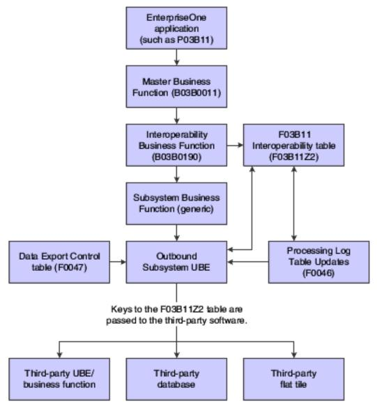
In this diagram, transactions are created in the Standard Invoice Entry program (P03B11) and sent through the outbound interoperability process to a third-party software package.
