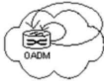
The small loop, which remains inside the network cloud, indicates that the component can be connected to the same component type in the same network system (intranetwork).
