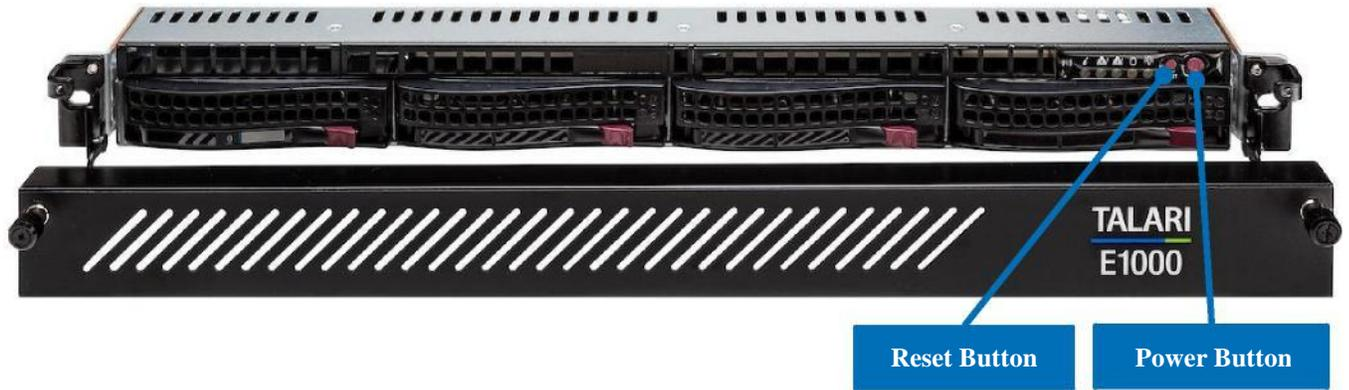
The Reset and Power buttons are located behind the faceplate of the appliance, and **should only be used under the direction of Talari Support**. To access the Reset or Power Buttons, the E1000 faceplate will need to be removed using the thumb screws:
