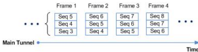
Figure 21-16 Redundancy — DTLS/UDP Redundancy
