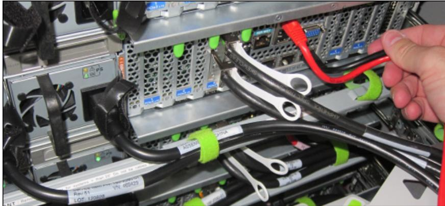
3. Route the cables through the CMA and secure them with hook and loop straps on both sides of each bend in the CMA.
