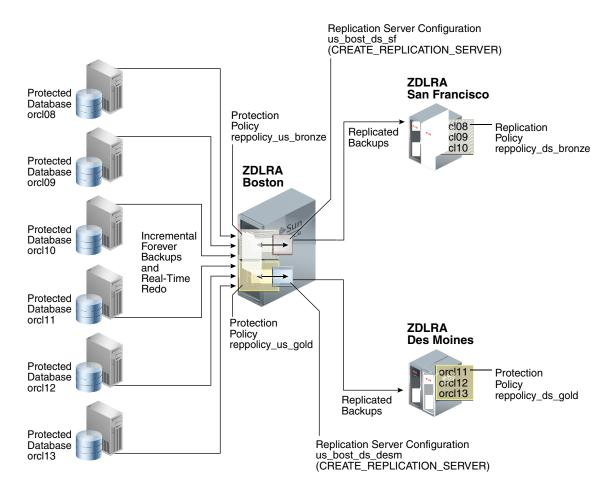
Figure 8-4 Different Protection Policies on Each Recovery Appliance
