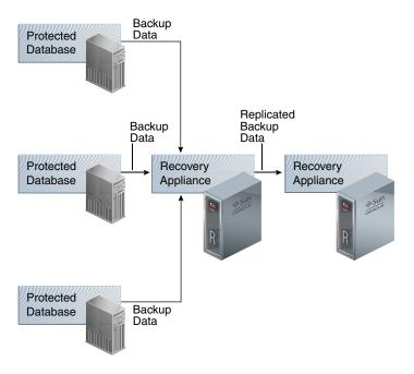
Figure 8-1 Simple Replication Topology
