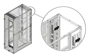
**Note -** For a 34KVA installation, connect the left VPS lower power cable to the HDPU1 connector, the left VPS upper power cable to the HPDU2 connector, the right VPS lower power cable to the HPDU3 connector, and the right VPS upper power cable to the HPDU4 connector.
