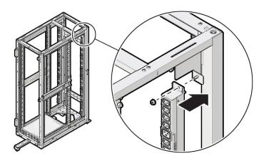
**Note -** For a 34KVA installation, connect the left VPS lower power cable to the HDPU1 connector, the left VPS upper power cable to the HPDU2 connector, the right VPS lower power cable to the HPDU3 connector, and the right VPS upper power cable to the HPDU4 connector.
