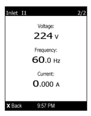
For a three-phase model, the next several pages show the unbalanced current percentage, line frequency, and the current and voltage values of each line.
