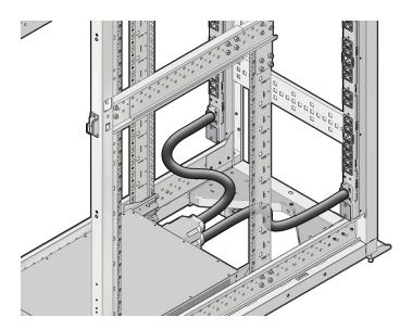
d. Slide the cable into the output connector, and secure it with M4 screws using a #2 Philips screwdriver, and torque to 15 in-lbs (1.7 Nm).
