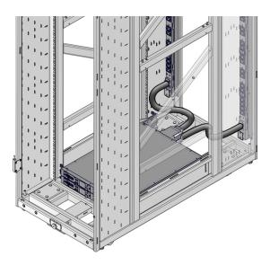
d. Slide the cable into the output connector, and secure it with M4 screws using a #2 Philips screwdriver, and torque to 15 in-lbs (1.7 Nm).
