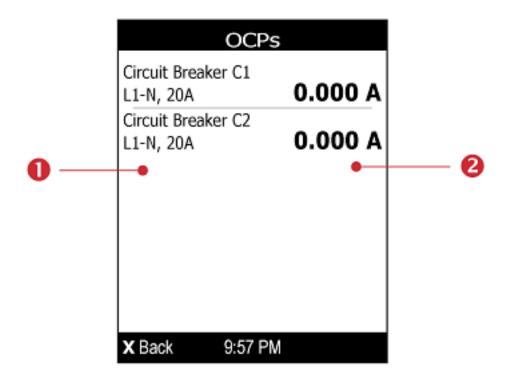
**Note -** If your HPDU model has multiple overcurrent protectors (OCPs) and appears on multiple pages, a page number appears in the upper-right corner of the top bar. Otherwise, no page numbers appear. If the overcurrent protector you want to view is not visible, press the Up or Down arrow buttons to scroll up or down.
