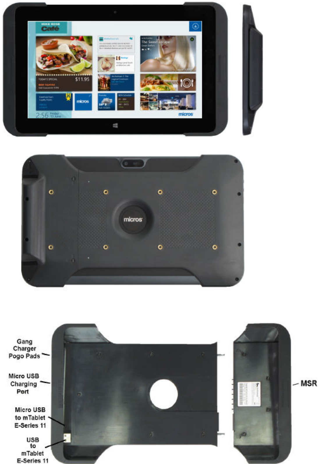
Figure 8-4 MICROS Tablet E-Series 11 with MSR Sleeve Features and Connectors
