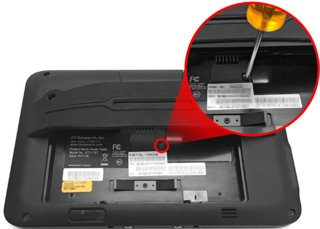
Figure 6-6 Removing the Bridge Battery Cover
