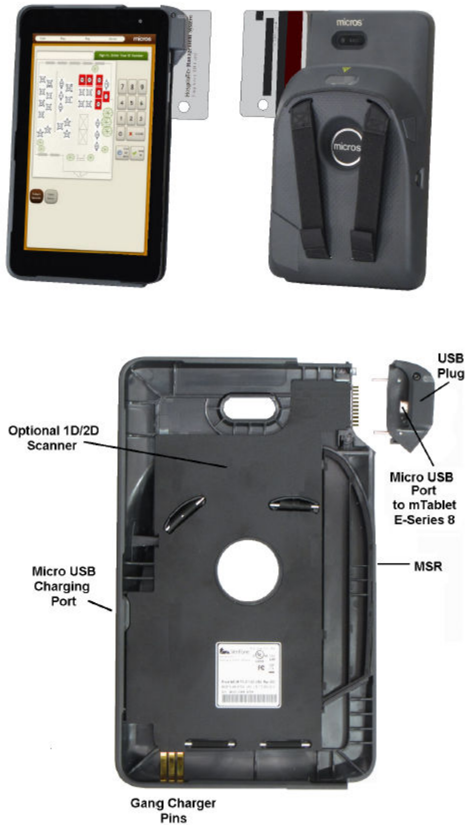
Figure 8-3 MICROS Tablet E-Series 8 with MSR Sleeve Features and Connectors
