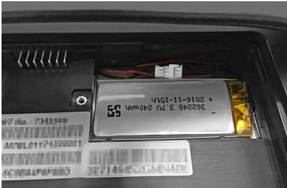
Figure 6-8 The Bridge Battery in the Battery Compartment
