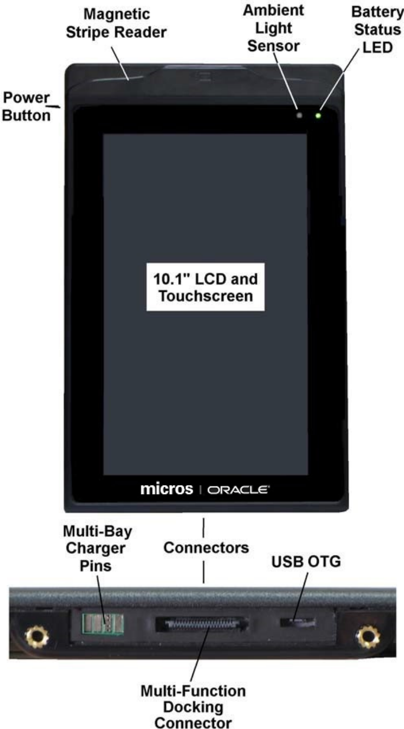
Figure 9-2 MICROS Tablet R-Series Features and Connectors
