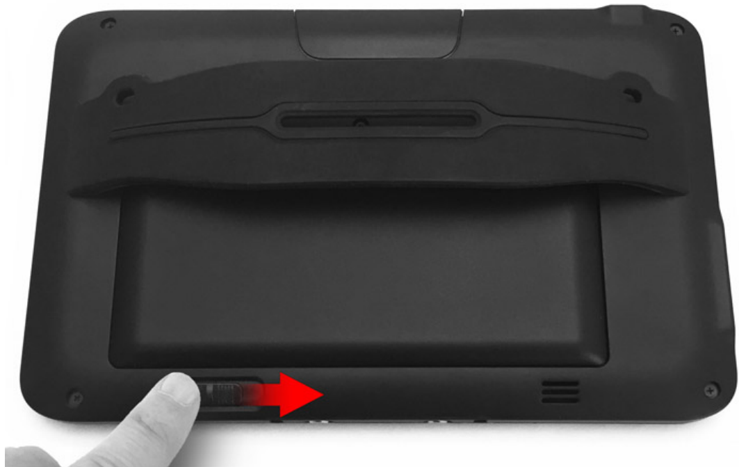
Figure 6-5 Removing the MICROS Tablet 720 Main Battery
