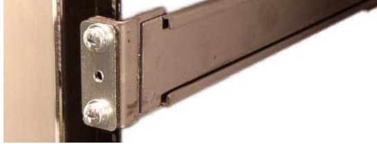
Figure 3 - 43. Installed Slide Rail in a Square-Hole Rack - Front Mount Point
