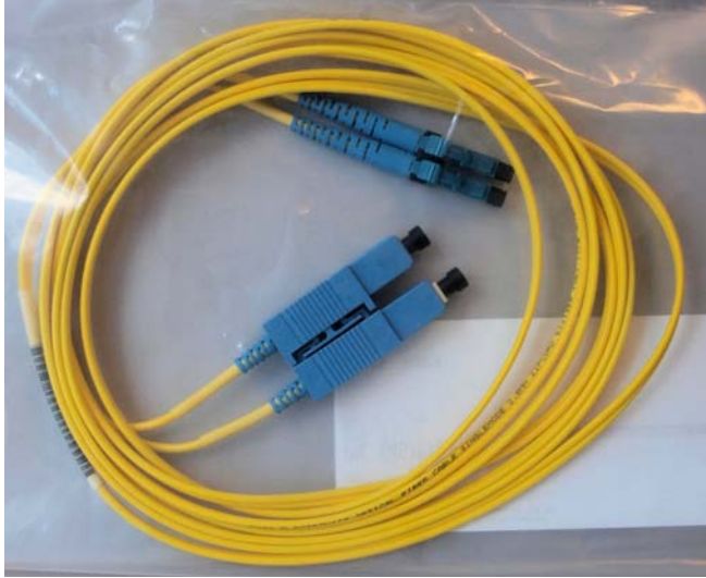
Figure 2 - 16. Single Mode LX Fiber Optic Cable
