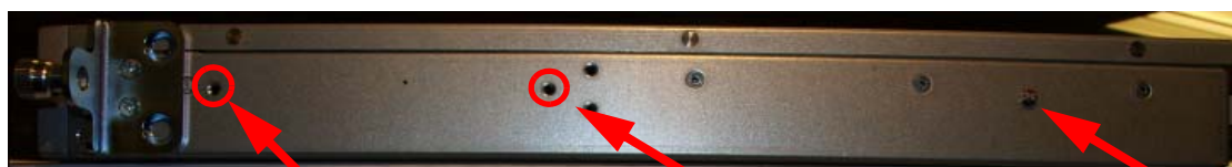
Tapped Chassis Holes for Slide Rail Holes #4 and #5
