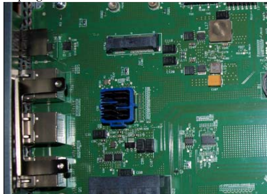
Figure 5 - 106. Internal view after T1/E1 TDM module removed
