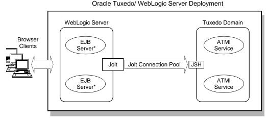
Figure 2-1 WebLogic Server to Oracle Tuxedo Connectivity Using Jolt
