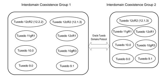
In this scenario, an Oracle Tuxedo domain (TDomain) gateway process running on a machine in one domain communicates over a network connection with a TDomain gateway process running on a machine in another domain. Table 1-1 lists the supported TDomain gateway processes.
