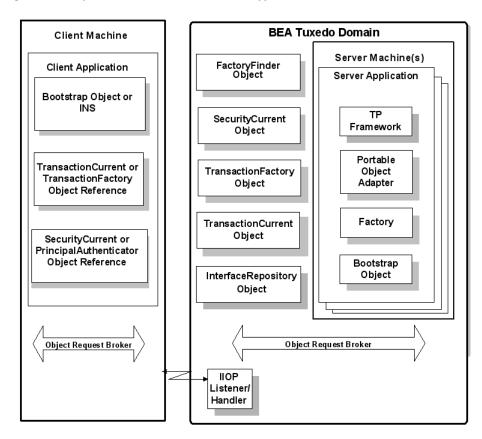
Figure 2-1 Components in a Oracle Tuxedo CORBA Application
