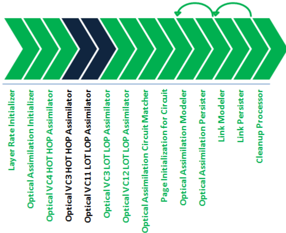
Figure 7-2 SONET Assimilation Processor Workflow
