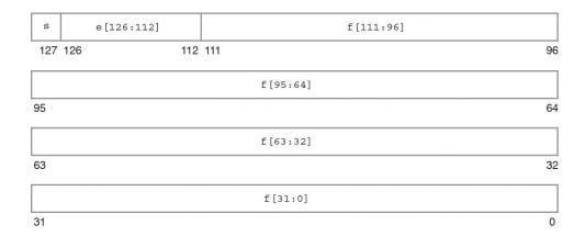
The values of the bit patterns in the three fields f, e, and s, determine the value represented by the overall bit pattern.
