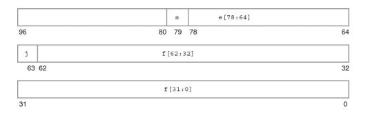
The values of the bit patterns in the four fields f, j, e and s, determine the value represented by the overall bit pattern.
