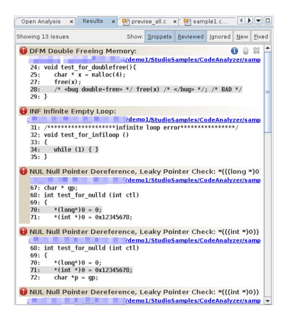
For each issue, the tab displays the issue type, the path name of the source file in which the issue was found, and a code snippet from that file with the relevant source line highlighted.
