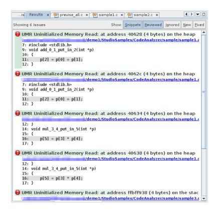
Look at the three issues that were added to the display and see how they are related to the core issues. Fixing the cause of the first issue in the display is likely also to eliminate the second and third issues. To hide the other dynamic memory access issues while you investigate the first one, click the Ignore button of the issues.
