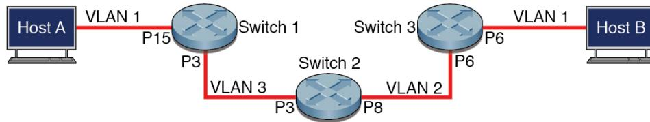
In this topology, P15, P3, P6, and P8 represent ports on the SEFOS switches. Switch 1 and switch 2 are NEM switches, and switch 3 is a TOR switch. The following table lists the IPv4 and IPv6 addresses of all the interfaces in both switches and the hosts.
