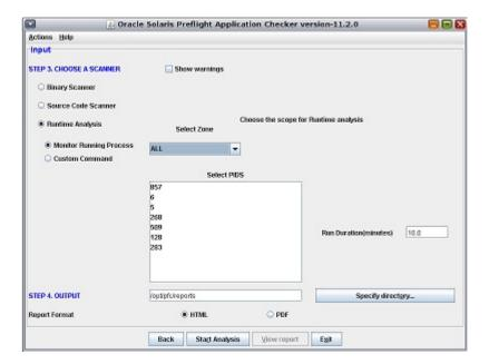
To analyze a user command, select the Custom Command option and type the complete command for starting the application to monitor the process.
