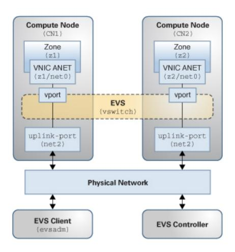
**FIGURE 5** Physical Components of an EVS Switch Configuration
