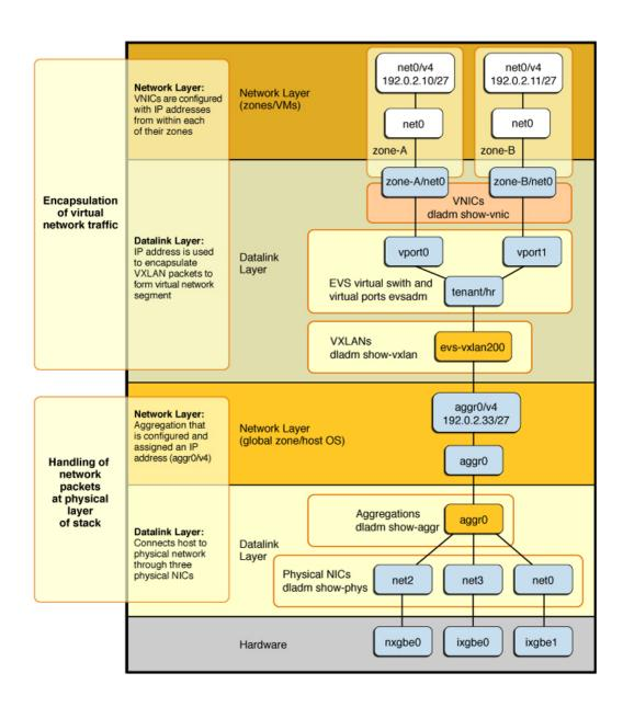
FIGURE 3 Combining Aggregations With VXLANs, VNICs, and an EVS Switch
