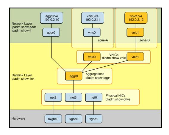
**FIGURE 2** Combining the Use of Aggregations With VNICs
