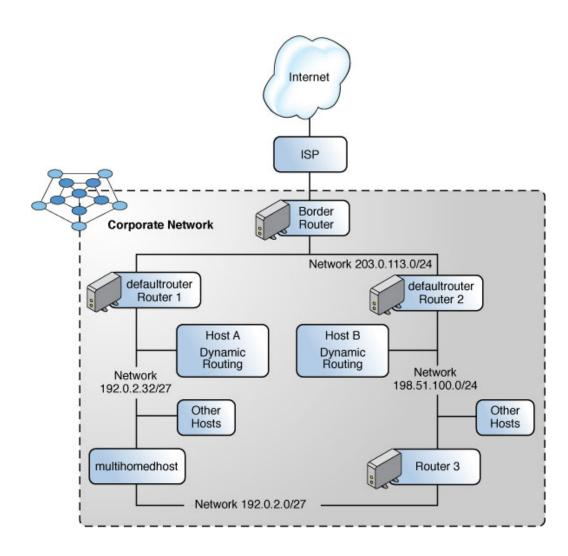
FIGURE 3 Autonomous System With Multiple IPv4 Routers
