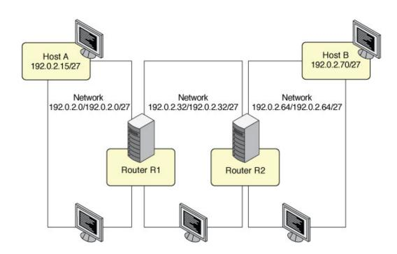
FIGURE 4 A Network Topology With Three Interconnected Networks
