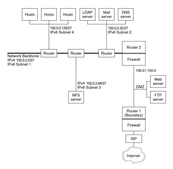
FIGURE 5 IPv6 Network Topology Scenario
