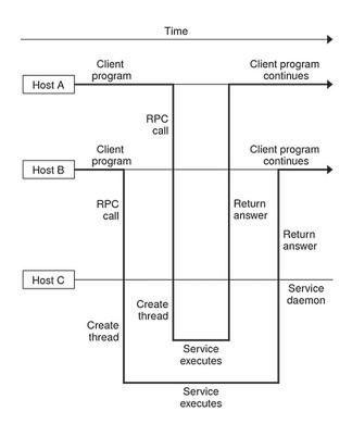
FIGURE 6 MT RPC Server Timing Diagram
