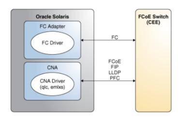
FIGURE 3 Connection With CEE-DCBX FCoE Switch by Using CNAs
