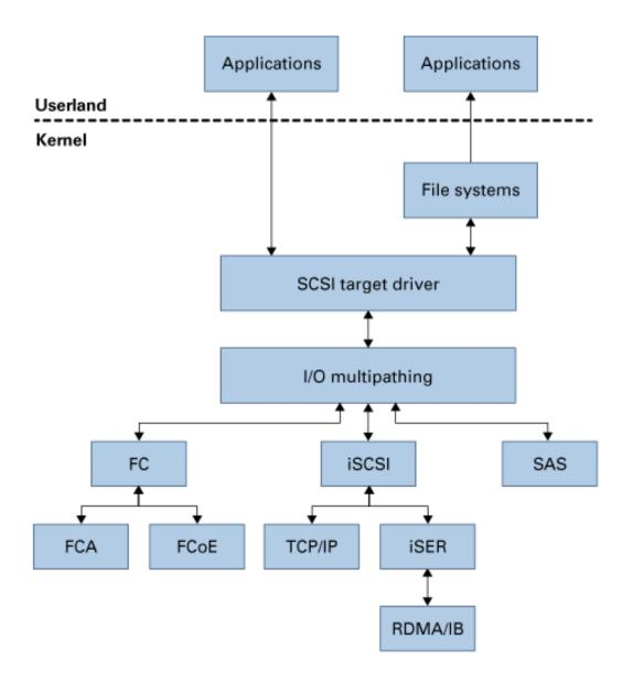
FIGURE 1 I/O Communication Between Oracle Solaris Storage Stack Components
