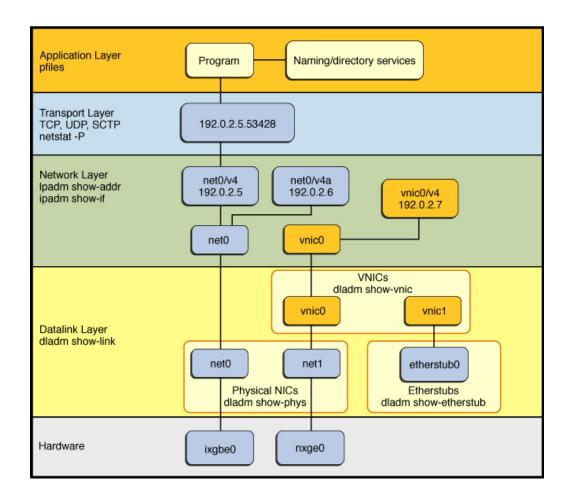
FIGURE 1 Oracle Solaris 11 Network Protocol Stack
