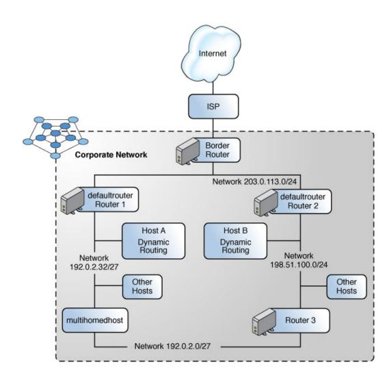
FIGURE 2 Autonomous System With Multiple IPv4 Routers
