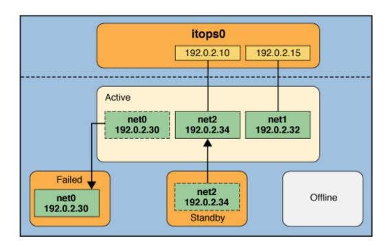
**Note -** The one-to-one mapping of data addresses to active interfaces in Figure 2, "Interface Failure in IPMP," on page 66 serves only to simplify the illustration. The IP kernel module can randomly assign data addresses without necessarily adhering to a one-to-one relationship between data addresses and interfaces.
