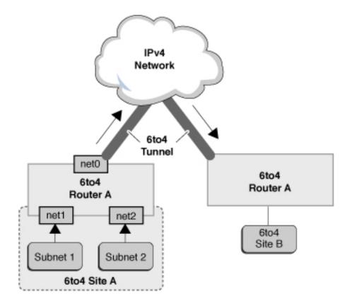
The previous figure depicts two isolated 6to4 networks, Site A and Site B. Each site has configured a router with an external connection to an IPv4 network. A 6to4 tunnel across the IPv4 network provides a connection to link 6to4 sites.
