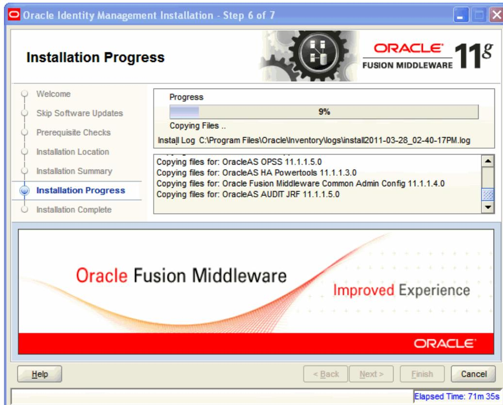
If you want to quit before the installation is completed, click **Cancel**. The installation progress indicator gives a running inventory of the files that are being installed. If you are only installing the software binaries, installation is complete after all of the binaries have been installed.
