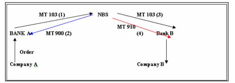
Once the PC transaction is booked and if the product is an RTGS product, the system processes the transaction in the following sequence:
