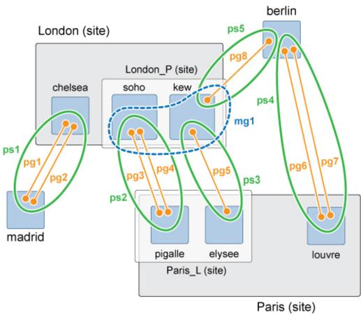
**FIGURE 3-4** Example Configuration of a Multigroup
