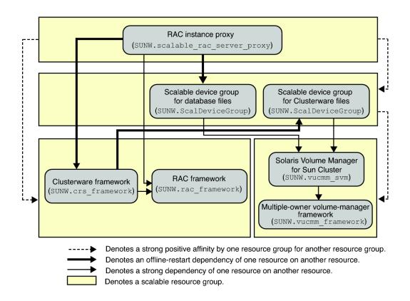
**FIGURE A-2** Configuration of Support for Oracle RAC With Solaris Volume Manager for Sun Cluster and Sun QFS Shared File System
