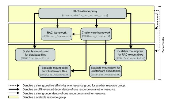
FIGURE A-10 Configuration of Support for Oracle RAC With a NAS Device in a Zone Cluster
