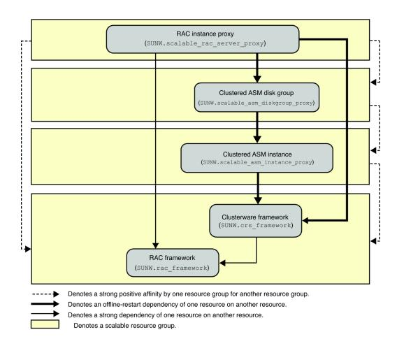
FIGURE A-6 Configuration of Support for Oracle RAC With Oracle ASM and Hardware RAID
