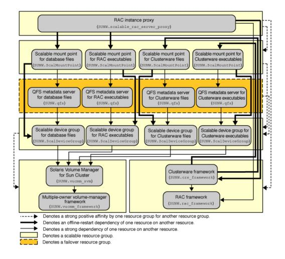
**FIGURE A-3** Configuration of Support for Oracle RAC With Sun QFS Shared File System and Hardware RAID
