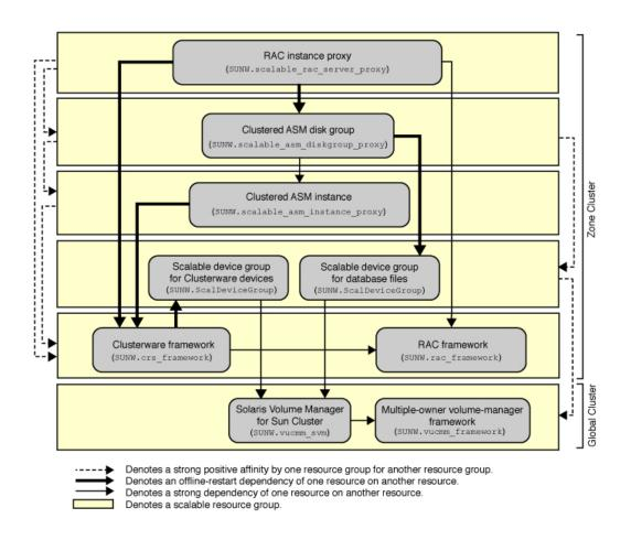
**FIGURE A-12** Configuration of Support for Oracle RAC With Oracle ASM and Hardware RAID in a Zone Cluster
