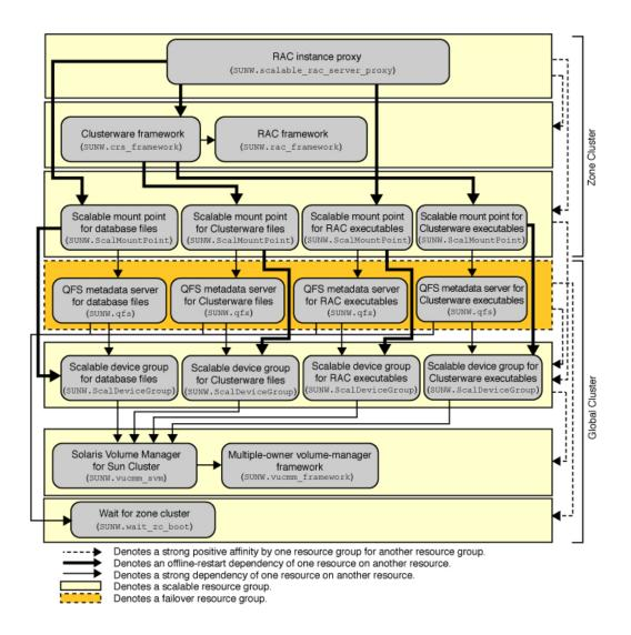
**FIGURE A-9** Configuration of Support for Oracle RAC With Sun QFS Shared File System and Hardware RAID in a Zone Cluster
