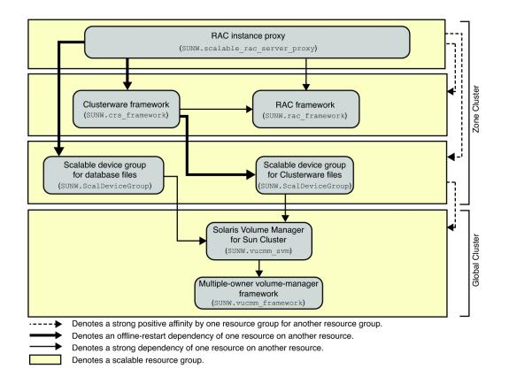
**FIGURE A-8** Configuration of Support for Oracle RAC With Solaris Volume Manager for Sun Cluster and Sun QFS Shared File System in a Zone Cluster
