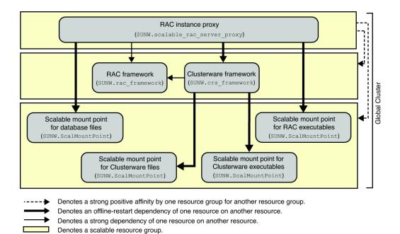
FIGURE A-4 Configuration of Support for Oracle RAC With a NAS Device
