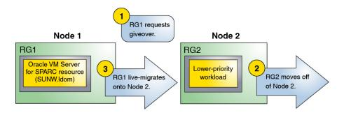
The giveover switches RG1 from Node1 to Node2, which results in eviction of resource group RG2 from Node2.
