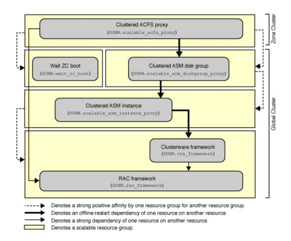
FIGURE 5-4 Configuration of Oracle ACFS in a Zone Cluster with Hardware RAID
