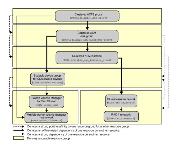
FIGURE 5-1 Configuration of Oracle ACFS in the Global Zone With Solaris Volume Manager
