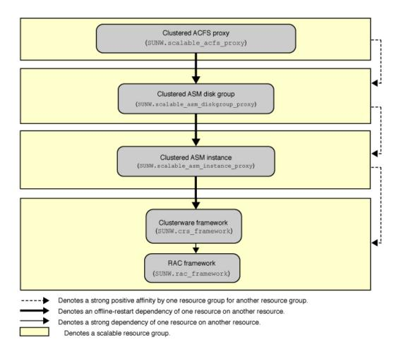
FIGURE 5-2 Configuration of Oracle ACFS in the Global Zone With Hardware RAID
