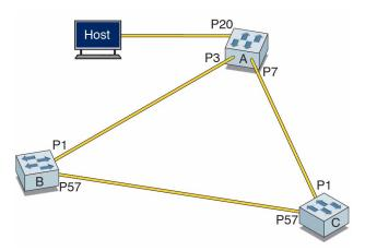
In this configuration, each switch A, B, and C, has two interfaces connected to the other two switches. Switch A has a third interface port 20 (P20) connected to a host. In addition to the default VLAN 1, VLAN 10 and VLAN 20 are used as command examples. The topology includes these details:
