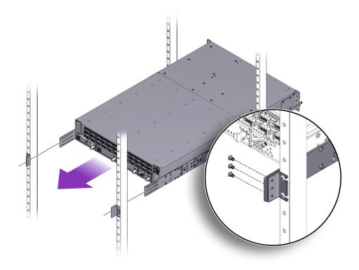
2. Keeping the Fabric Interconnect level, insert the appropriate rack mounting screws (10-32, 12-24, or M6) into the mounting brackets on the front of the Fabric Interconnect (the fan unit end). See Figure 27, "Securing the Front Mounting Brackets to the Equipment Rack," on page 54.
