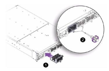
When the fan module is almost all the way inserted, you might feel some resistance, which is caused by the fan module's power socket meeting its mating part. Continue to apply gentle pressure until the fan module is fully seated in the Fabric Interconnect F1-4 chassis. The fan module is correctly seated when the fan module sits flush with the face of the Fabric Interconnect F1-4.
