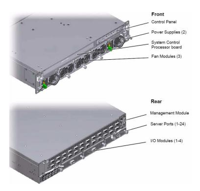
The Fabric Interconnect F1-4 can also support InfiniBand connections at Quad Data Rate (QDR) speeds. Figure 33, "QDR Fabric Interconnect F1-4 Rear Panel Components," on page 61 shows the Fabric Interconnect F1-4's rear panel with a QDR Fabric Board installed. The QDR Fabric Board is easily identifiable by the different layout of its 20 physical ports.
