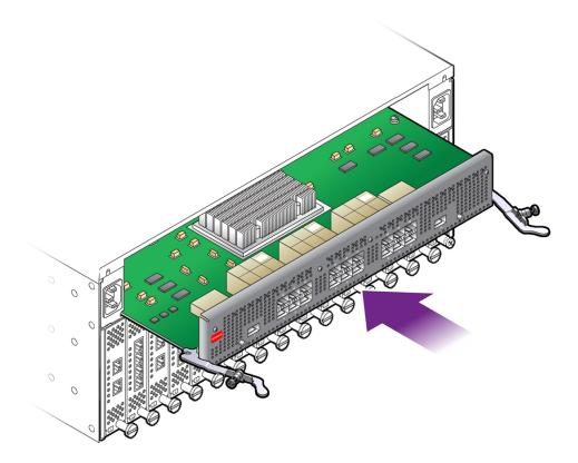
9. When the Fabric Board is properly aligned, gently slide it in until you feel some resistance, then check the notches at the end of the Fabric Board's handles to make sure they are contacting the guides on the inside of the chassis.
