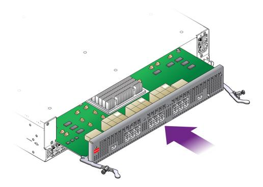
9. When the Fabric Board is properly aligned, gently slide it in until you feel some resistance, then check the notches at the end of the Fabric Board's handles to make sure they are contacting the guides on the inside of the chassis.
