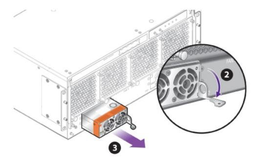
3. Use the finger hole in the locking lever to remove the power supply from the chassis (3).
