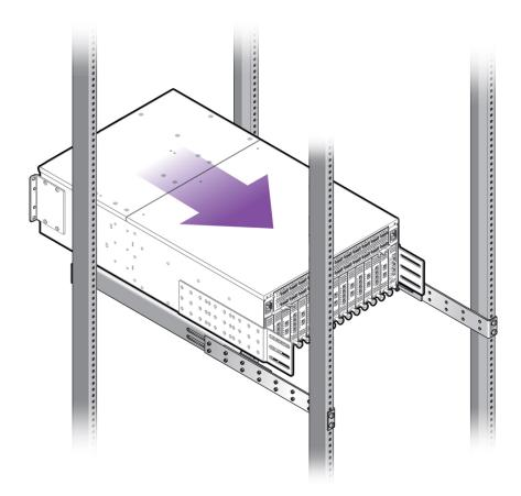
**Note -** Figure 10, "Inserting the Fabric Interconnect F1-15 into the Equipment Rack," on page 30 shows installing the Fabric Interconnect from the rear of the rack. Whether you install back-to-front, as shown, or front-to-back is irrelevant as long as the chassis is inserted so that it is supported on the horizontal surface of the rails. The horizontal surface is required to support the Fabric Interconnect as it slides into the rack.
