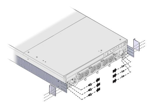
**FIGURE 28** Aligning the Angle Brackets and Inserting the Screws
