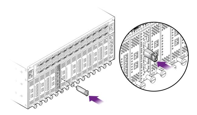
4. Insert one end of the optical cable into the SFP+ transceiver. See Figure 54, "Inserting the Optical Cable into the Optical Transceiver," on page 85.
