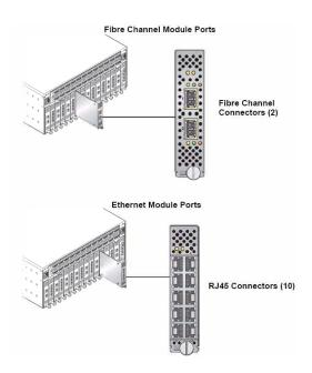
Figure 51, "Fabric Interconnect F1-15 Fibre Channel and Gigabit Ethernet Modules and Connectors," on page 81 shows an example of the 10-Port GE module, but the 10 GE module (which has one 10 GE port) is also supported.
