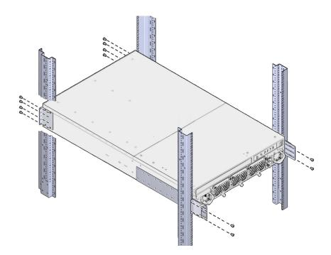
6. With the chassis adjusted to your preferred rack depth, tighten the M3.5 screws.
