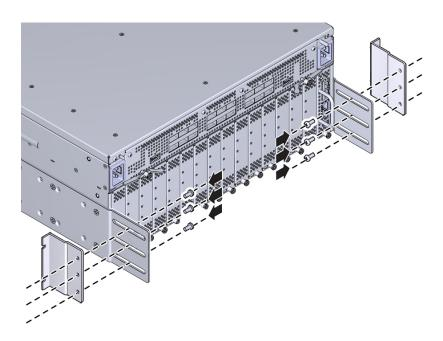
Make sure the screw holes in the angle brackets lie flush against the slotted edge of the side panels. The slotted edge of the angle bracket will attach to the rack post.
