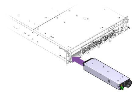
When the PSU is almost all the way inserted, you might feel some resistance, which is caused by the PSU's power socket meeting its mating part on the Fabric Interconnect F1-4 midplane. Continue to apply gentle pressure until the PSU is fully seated in the Fabric Interconnect F1-4 chassis.
