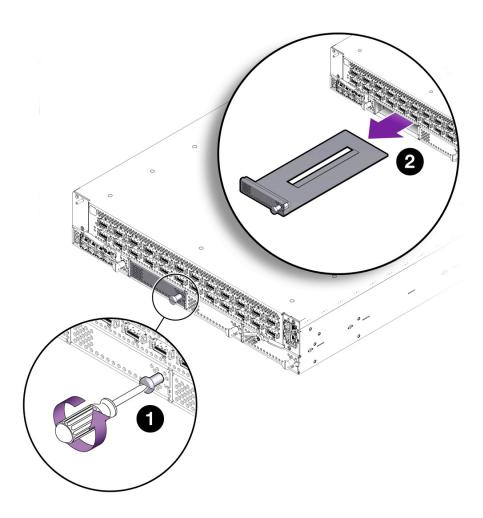
4. Grasp the module handle and remove the I/O module, while keeping the module level (2) as shown in Figure 93, "Removing a Fabric Interconnect F1-4 I/O Module," on page 145.
