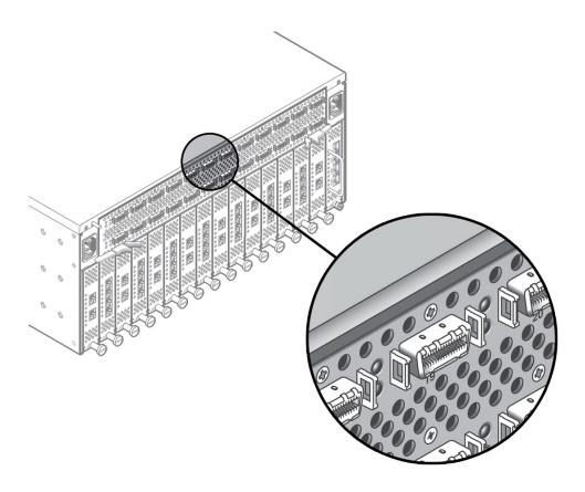
Figure 50, "InfiniBand Ports for Fabric Interconnect F1-4 Client Server Connections," on page 80 shows an InfiniBand port connection on the Fabric Interconnect F1-4 with a DDR Fabric Board.
