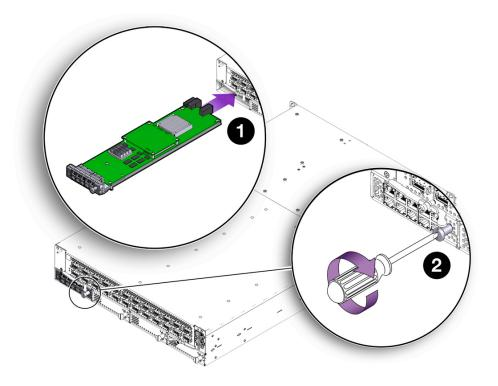
When the I/O Module is almost completely inserted, you will feel some resistance, which is the I/O Module's connector meeting its midplane socket. Continue to apply gentle pressure until the connector is seated in the socket.
