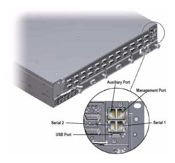
There are two ways to connect to the serial port on the Fabric Interconnect Management module:
