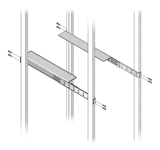
16. When the rails are attached to the rack posts, tighten all screws that connect the pieces of the rail, as well as the screws that attach each assembled rail to the rack.
