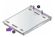
**Note -** Some servers have a different method of securing the cover to the server. For example, some servers have a securing screw at the rear of the server that holds the cover in place. If your server's cover is held in place by a different method than the illustration shows, consult the manufacturer's documentation for the correct way to remove the cover.
