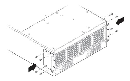
This illustration shows new mounting bracket installation for an Oracle Fabric Interconnect F1-15. For an Oracle Fabric Interconnection F1-4, see "Install a Fabric Interconnect F1-4 Front Panel Assembly" on page 155.
