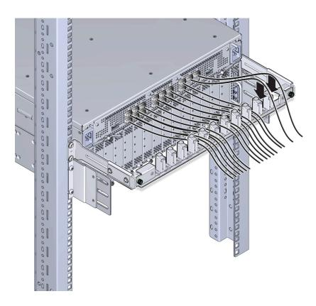
14. When all cables are connected, align the captive screws in the top of the CMA with the screw holes in the CMA's comb as shown in Figure 21, "Installing the Top of the CMA," on page 44.
