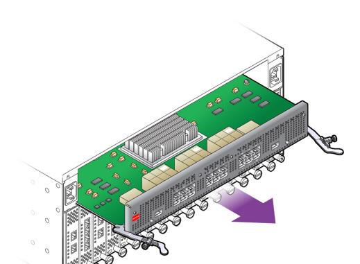
FIGURE 76 Removing the Fabric Interconnect F1-15 QDR Fabric Board
