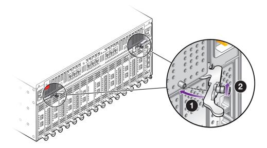
When the release levers have correctly locked the QDR Fabric Board into the chassis, use the screwdriver to secure the captive screws in the release levers (2).
