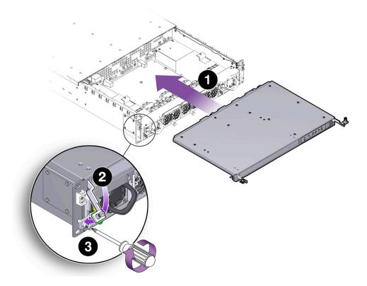
As the Front Panel slides into place, you will feel the gaskets at the rear of the Front Panel make contact with the chassis sheet metal.
