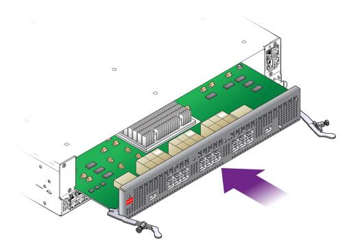
11. When the Fabric Board is properly aligned, gently slide it in until you feel some resistance, then check the notches at the end of the Fabric Board's handles to make sure they are contacting the guides on the inside of the chassis.
