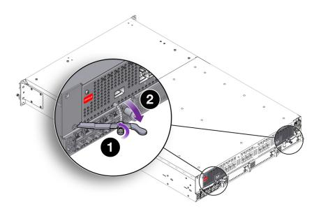
4. When the screws are loose, grasp the Fabric Board's handles and simultaneously pivot them outward (2) as shown in Figure 79, "Unlocking the Fabric Interconnect F1-4's Fabric Board," on page 124. The handles act as levers that disconnect the Fabric Board from the Fabric Interconnect F1-4 midplane. As a result, you might encounter some resistance when you first apply pressure to pivot the handles outward.
