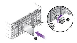
Secure the module in the slot by tightening the securing screw (2), located at the bottom edge of the module's rear panel.
