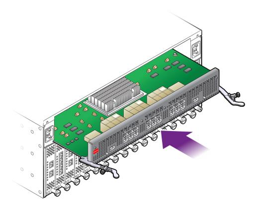
11. When the Fabric Board is properly aligned, gently slide it in until you feel some resistance, then check the notches at the end of the Fabric Board's handles to make sure they are contacting the guides on the inside of the chassis.
