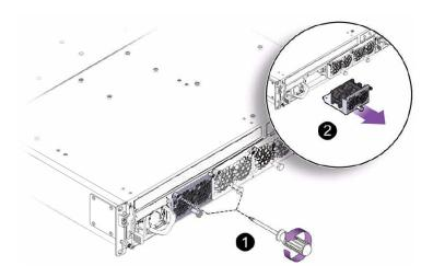
2. Grasp the handle and slide the fan module out of the chassis (2).
