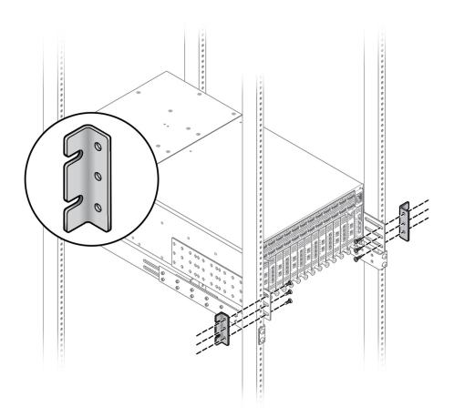
3. When the angle brackets are installed on the side panel, insert the pan-head screws (10-32, 12-24, or M6) through the slotted edge of the angle bracket, into the chassis and tighten the screws to attach the chassis to the rack. Each point of attachment to the rack requires two screws. Figure 12, "Attaching the Chassis to the Rack Posts," on page 33 shows attaching the chassis to the rack.
