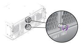
2. Grasp the handle and slide the fan module out of the chassis. See Figure 62, "Removing a Fabric Interconnect F1-15 Fan Module," on page 104.
