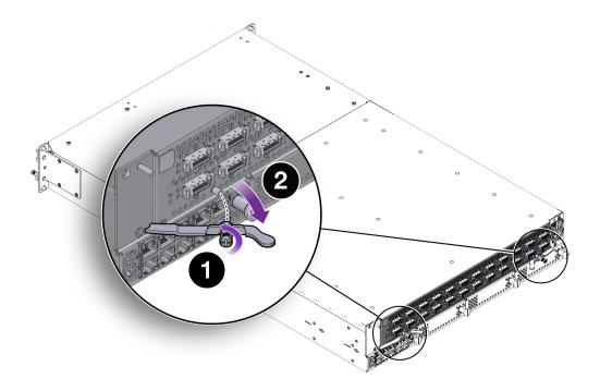
4. When the screws are loose, grasp the Fabric Board's handles and simultaneously pivot them outward (2) as shown in Figure 71, "Unlocking the Fabric Interconnect F1-4's Fabric Board," on page 115. The handles act as levers that disconnect the Fabric Board from the Fabric Interconnect F1-4 midplane. As a result, you might encounter some resistance when you first apply pressure to pivot the handles outward.
