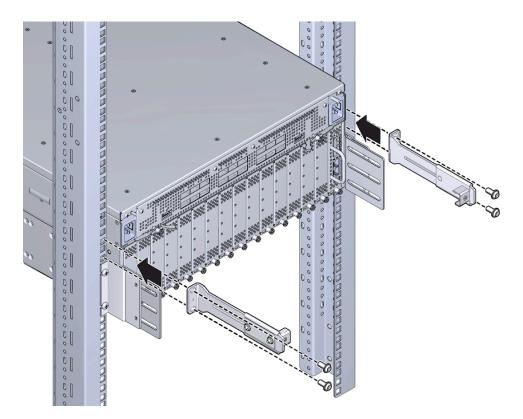
**FIGURE 18** front brackets being installed
