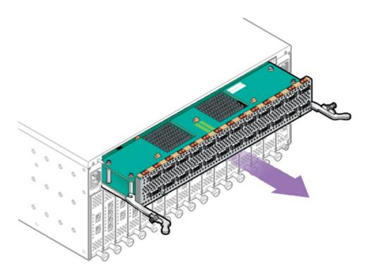
**FIGURE 84** Removing the DDR Fabric Board from a Fabric Interconnect F1-15
