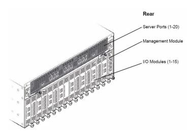
Figure 32, "Fabric Interconnect F1-4 Front and Rear Panel Components," on page 60 shows the Fabric Interconnect F1-4's chassis components on the front and rear panels. The following illustration shows an InfiniBand Fabric Interconnect F1-4 supporting DDR connectivity.
