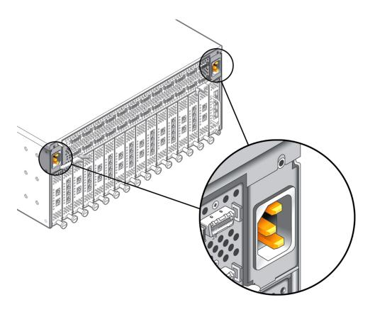
2. On the opposite side of Oracle Fabric Interconnect, simultaneously switch all power supplies to the "On" position.
