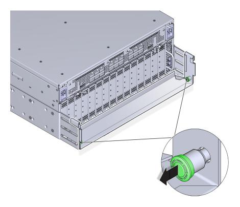
7. Simultaneously pull the two pins inward (toward each other), and slide the module retention bracket off of the Fabric Interconnect chassis. See Figure 6, "Removing the Module Retention Bracket," on page 25.
