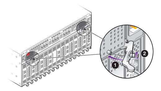
13. When the release levers have correctly locked the QDR Fabric Board into the chassis, use the screwdriver to secure the captive screws in the release levers (2).
