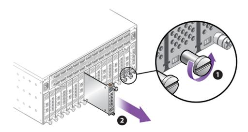
4. Grasp the locking handle (2) and slide the module out of the chassis.
