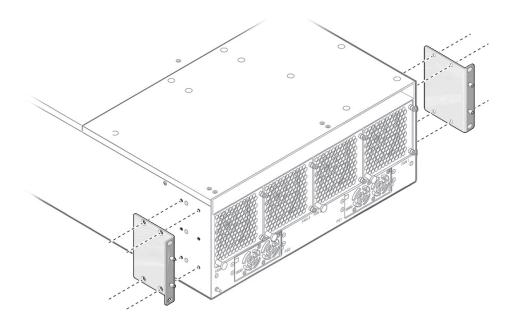
2. Insert and tighten the screws to attach the new mounting brackets to the chassis.
