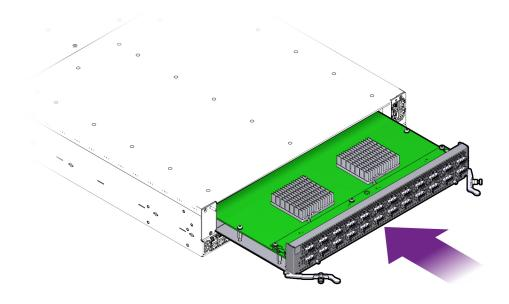
When the Fabric Board is almost completely inserted, you will feel some resistance when the connector at the rear of the Fabric Board contacts its socket on the inside of the chassis.
