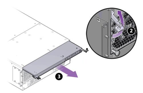
**FIGURE 97** Removing the Fabric Interconnect F1-15 Front Panel Assembly
