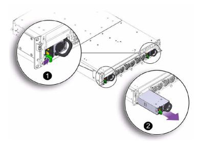
**Note** - Both PSUs are oriented in the same direction, so both locking tabs pull to the right.
