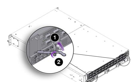
FIGURE 74 Securing the Fabric Interconnect F1-4's Fabric Board
