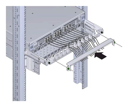
15. Using a Phillips-head screwdriver, tighten the screws to secure the plate to the comb as shown in Figure 22, "Completing Assembly of the CMA," on page 45.
