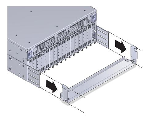
**Note -** The module retention bracket is used to hold modules and blanks in place while the product is in transit. After removing the module retention bracket, keep it for future use.
