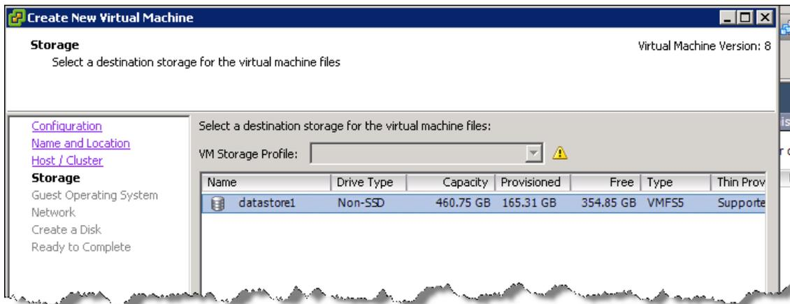
Figure 11 Selecting storage for the Virtual Machine
