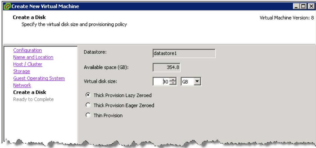
Figure 14 Specifying the Virtual Machine's Size
