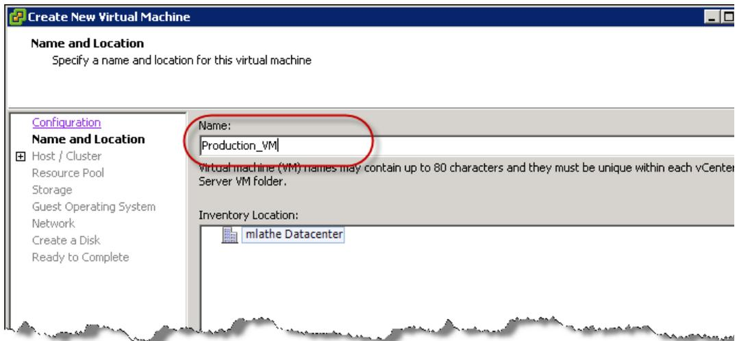
Figure 9 Specifying the Virtual Machine Name
