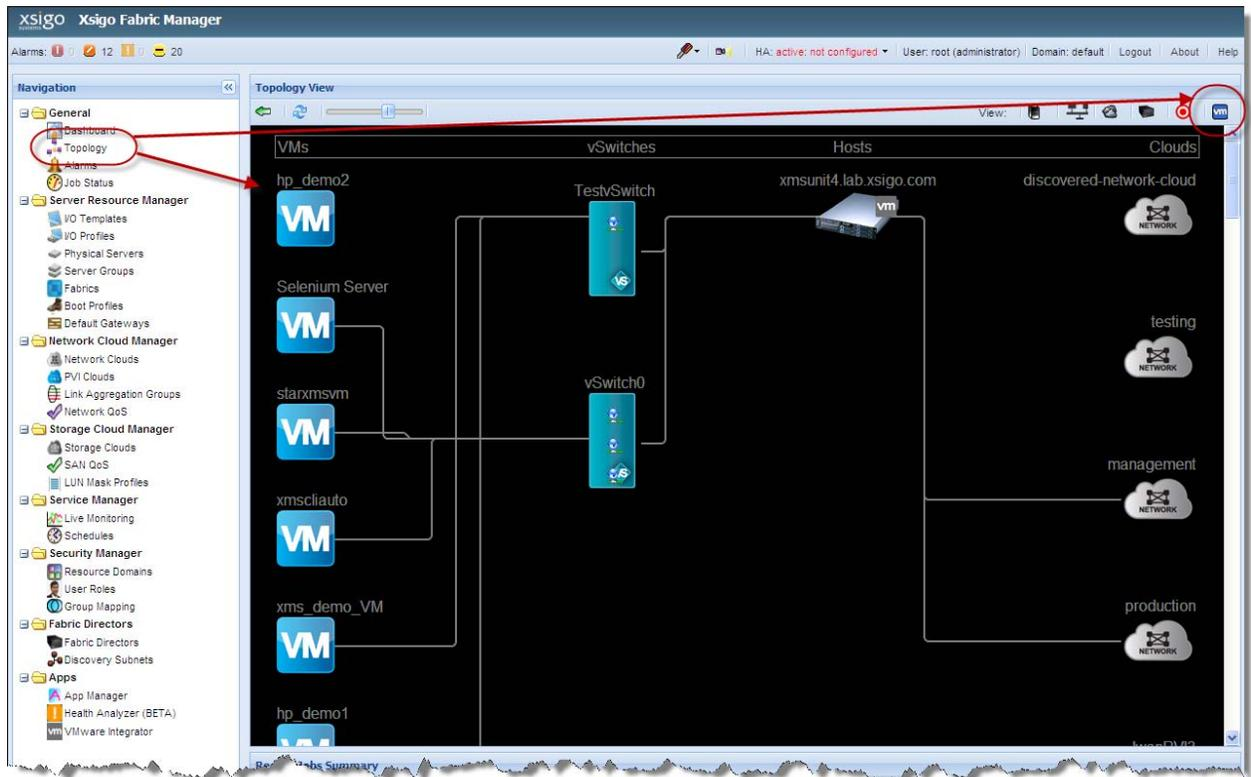
Figure 10 Virtual Machine and vSwitch Topology View
