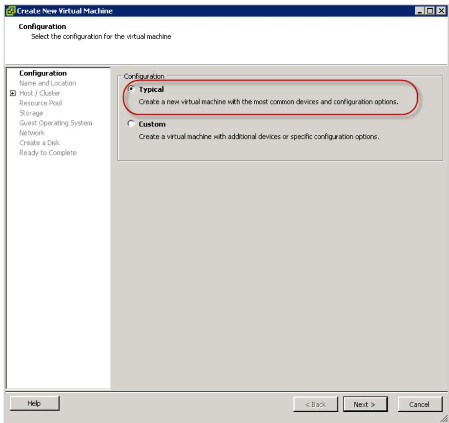
Figure 8 Creating a *Typical* Virtual Machine
