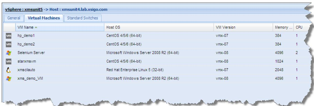
Figure 4 Virtual Machines Discovered by Fabric Manager
