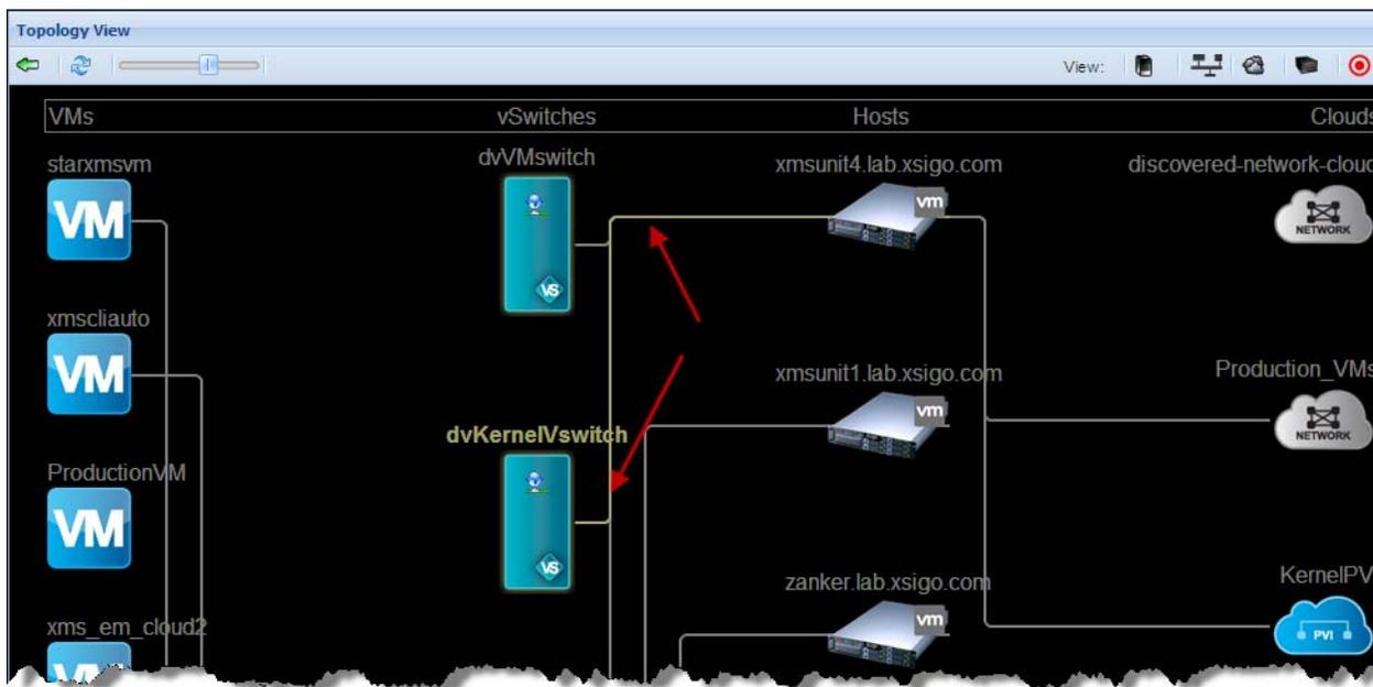
Figure 4 Connection Lines in Topology View
