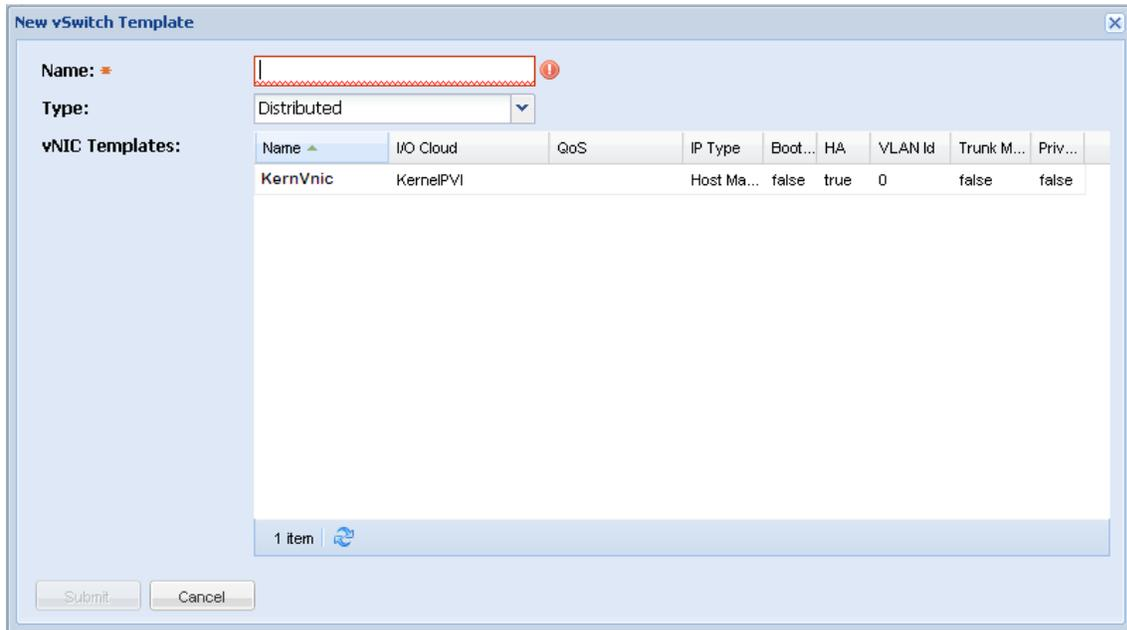
Figure 27 Adding a New Distributed vSwitch
