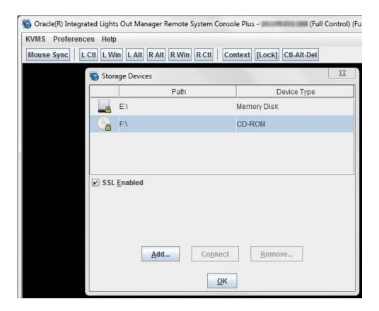
**Note -** The Storage Device dialog box automatically displays storage drive devices (such as CD, DVD, floppy, and USB devices) detected on the Oracle ILOM Remote Console Plus client. If bootable media is not detected in the drive, a lock icon appears on the drive to indicate: 1) the drive is present, and 2) bootable media was not found in the drive.
