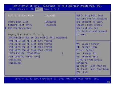
6. In the Boot menu, verify that the UEFI/BIOS Boot Mode is set to the appropriate value for your installation.
