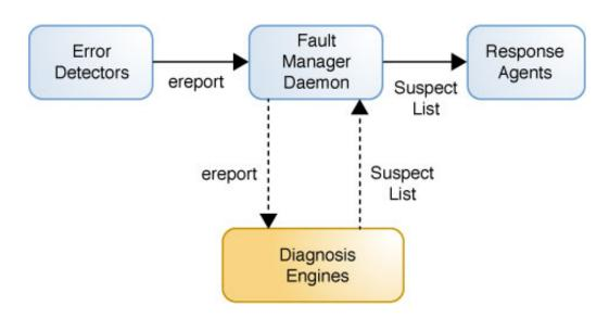
**FIGURE 1-1** Fault Management Architecture Components
