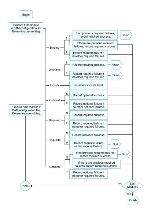
FIGURE 1-2 PAM Stacking: Effect of Control Flags
