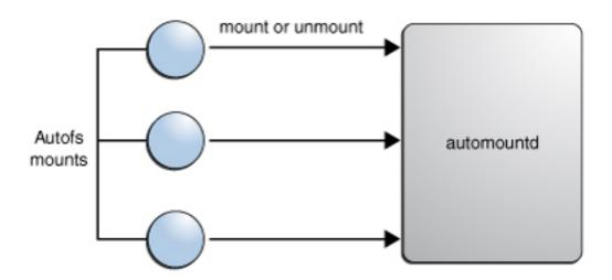
After the autofs mounts are set up, these mounts can trigger file systems to be mounted under them. For example, when autofs receives a request to access a file system that is not currently mounted, autofs calls automountd, which actually mounts the requested file system.
