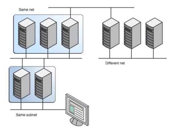
If several servers that support the same protocol are on the local subnet, the time to connect to each server is determined and the fastest server is used. The sorting can also be influenced by using weighting. For more information about weighting, see "Autofs and Weighting" on page 61.
