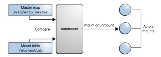
This figure shows that automount compares entries in the master map with entries in the mount table to generate a current list.
