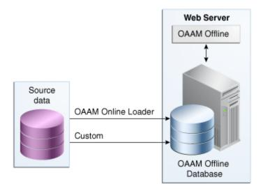
OAAM Offline has its own database. This database has an identical schema to that of the OAAM Online version. It is used to load customer data to perform risk analysis and tune rules. OAAM Offline can support both login and transaction data. For information on the types of loaders that are used to load data, refer to Section 22.1.7, "Data Loaders."
