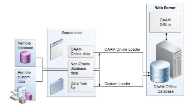
The standard OAAM Loader, which is shipped with OAAM, can be used to load login data from an OAAM schema database or a remote database that is mapped to the OAAM schema.
