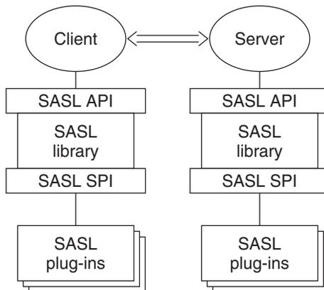
Client and server applications make calls to their local copies of `libsasl` through the SASL API. `libsasl` communicates with the SASL mechanisms through the SASL service provider interface (SPI).
