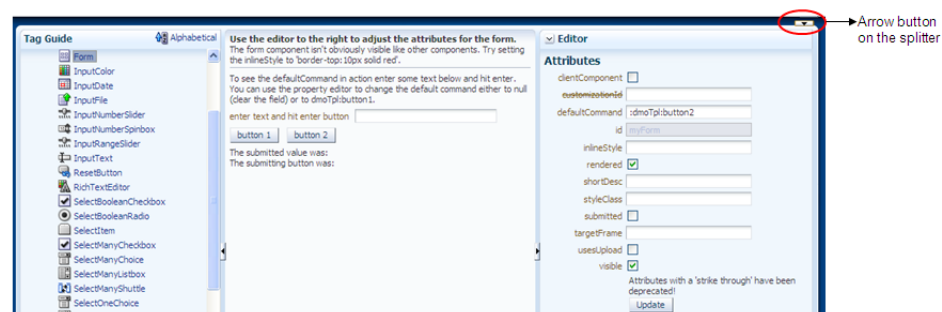
Figure 9–12 panelSplitter with a Vertical Split Collapsed
