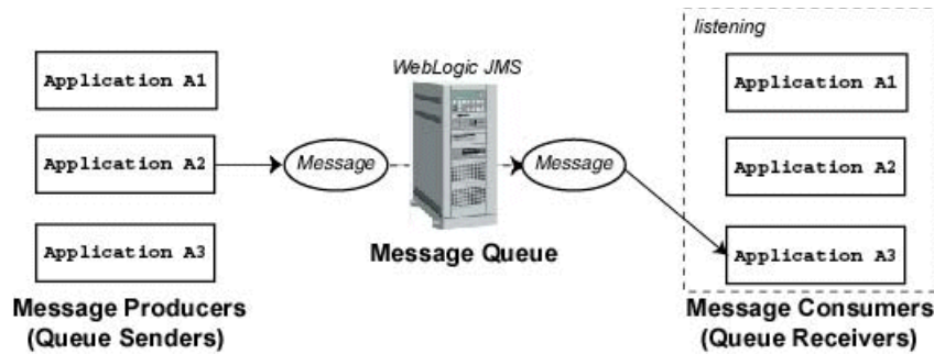
Figure 2–3 Point-to-Point (PTP) Messaging
