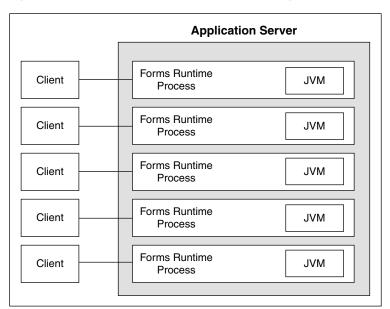
Figure 10–2 Forms Runtime with no JVM Pooling
