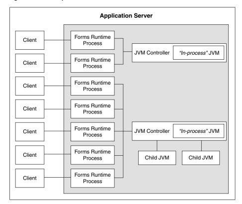
Figure 10-1 Multiple JVM Controllers with Child Processes
