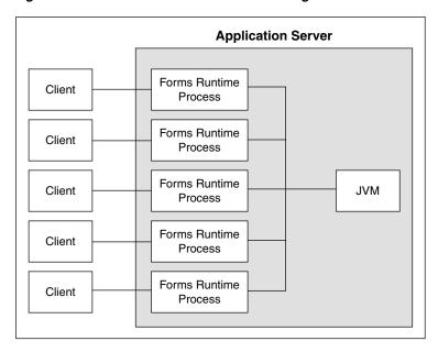
Figure 10–3 Forms Runtime with JVM Pooling Enabled
