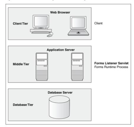
Figure 2-2 Three-tier configuration for running a form
