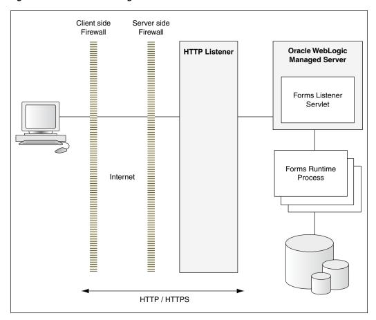
Figure 2-3 Architecture using the Forms Listener Servlet
