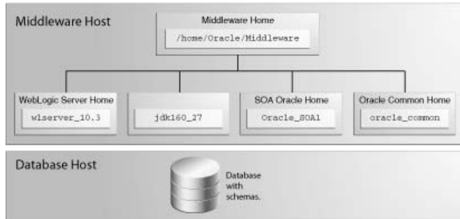
Figure 4 Directory Structure After Oracle SOA Suite Installation
