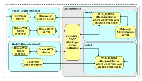
Figure 6–2 Discoverer topology for a multiple-instance environment
