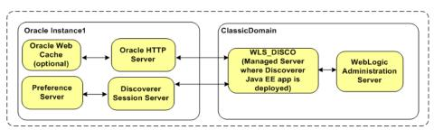
Figure 6–1 Discoverer topology for a single instance
