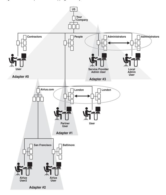
Figure 2–11 Example of an Overlapping Directory Structure
