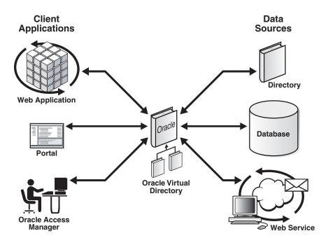
Figure 1–1 Oracle Virtual Directory Clients and Connectable Data Stores
