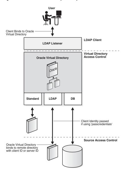
Figure 6-1 Oracle Virtual Directory Multi-Layered Access Control and Authentication
